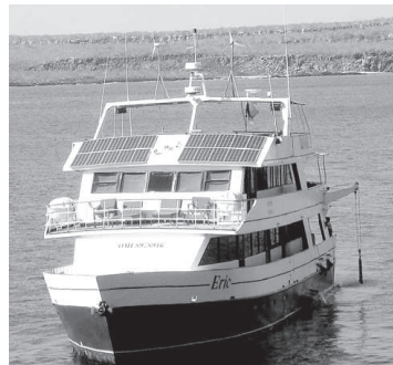
Eric, this 67-foot boat, boasts 40 solar panels and two wind turbines.
